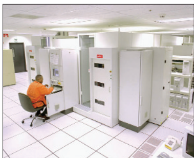
Two "farms" of PCs at Fermilab. Such clusters have largely replaced multiprocessor mainframes.
